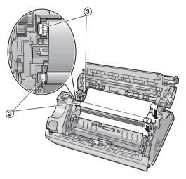
**5** Turn the blue gear (④) in the direction of the arrow until the ink film is tight (⑤) and at least one layer of ink film is wrapped around the blue core (⑥).
